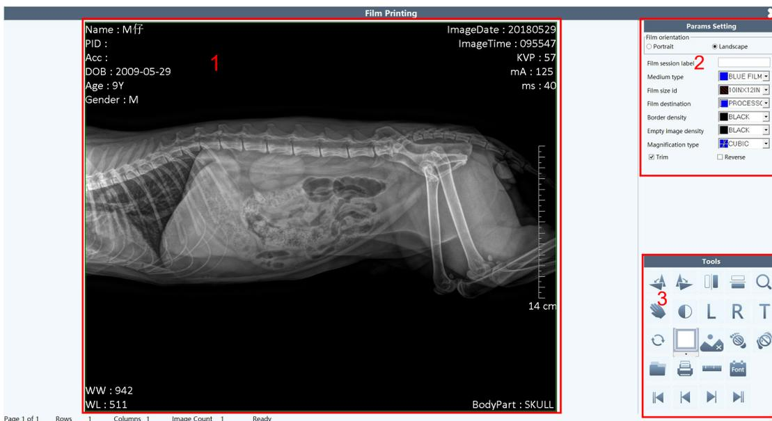
Here, [1] indicates the image preview pane, [2] indicates the **Params Setting** pane, and [3] indicates the image processing tool pane.
